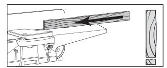
**4. Rip Cut On A Table Saw**—The jointed edge of the workpiece is placed against a table saw fence and the opposite edge cut off.
